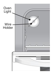
The oven light automatically turns ON when the door is opened. The oven light may also be manually operated by pressing the oven light switch located on top of the control panel.
